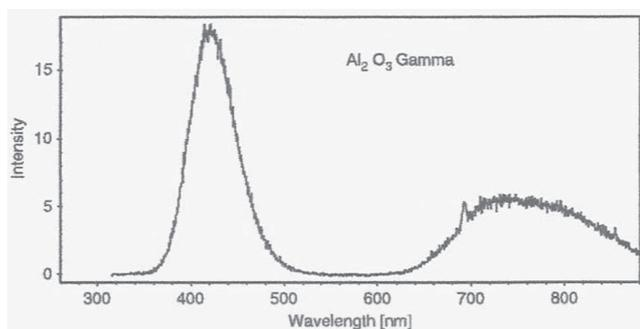
**Figure 3.** Thermoluminescent spectrum of  $\alpha$ - $\text{Al}_2\text{O}_3$  at 235–242 K after gamma-ray irradiation. The strongest peak appears at about 420 nm, in addition to another at 730 nm (Koike et al. 2006).
