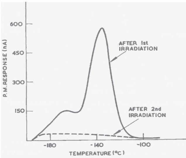
**Figure 5.** Thermoluminescent glow curves of pale pyroxene fraction, in the range 435–485 nm (Blair & Edgington 1970).
