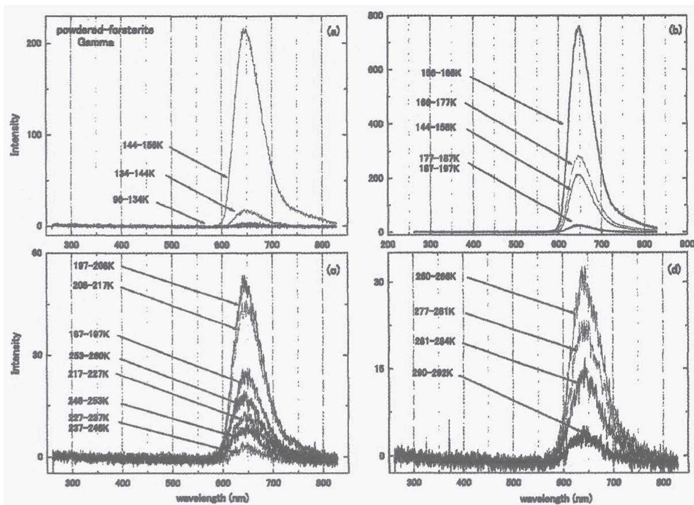
**Figure 2.** Thermoluminescent spectra of powdered forsterite. The warming temperature increases from panels (a) to (d). The intensity becomes stronger at 144–177 K and strongest at 156–166 K, but the intensity suddenly grew weak at higher temperature (Koike et al. 2002a).
