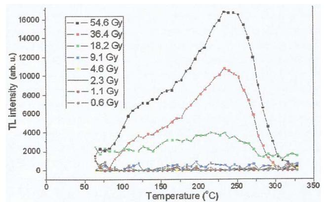
**Figure 4.** Thermoluminescent glow curve of CVD diamond samples exposed to 0.6–55 Gy gamma irradiation doses (Karczmarzka et al. 2012).
